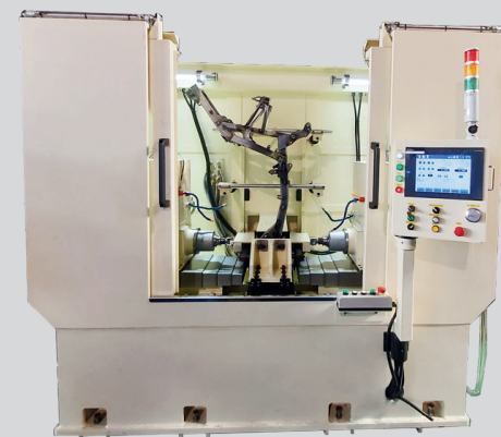
2 Ways Fine Boring Machine FBHDS41
